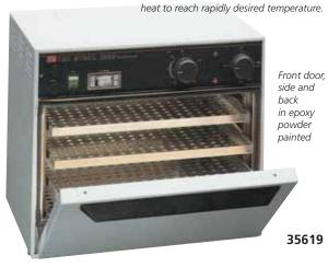
**TECHNICAL SPECIFICATIONS TAU 1.6** TAU 6 **TAU 18** 385x170xh 90 375x230xh 200 Inside dimensions (mm): 245x115xh 55 Outside dimensions (mm): 310x180xh 180 495x310xh 220 440x310xh 380 Weight: 5 kg 10.5 kg 14 kg Operating voltage: 220 V 220 V 110V available on request 250 W 600 W 400 W Power consumption: 3.15 A Fuses: Thermostat: Automatic capillary bulb type with self registration from 90° to 200° Timer: from 0 to 120 minutes high precision with capillary bulb Thermometer: Made in Italy
